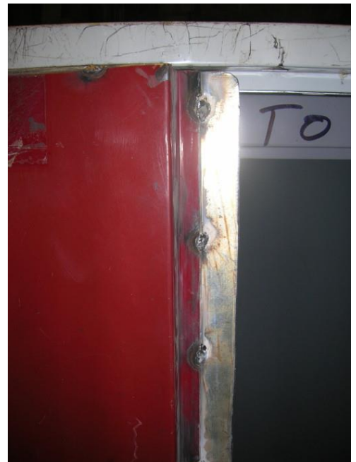
I left the skin wide on one door so the doors had a bigger overlap in the middle
