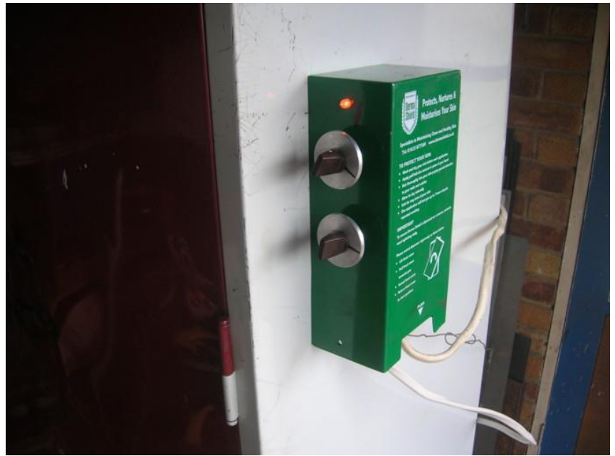
A steel industrial soap dispenser (from a skip) as my control box
