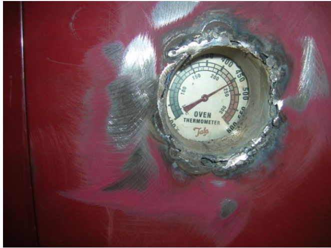
An oven thermometer shows the temp. I know the welding's crap, my mig's playing up.
