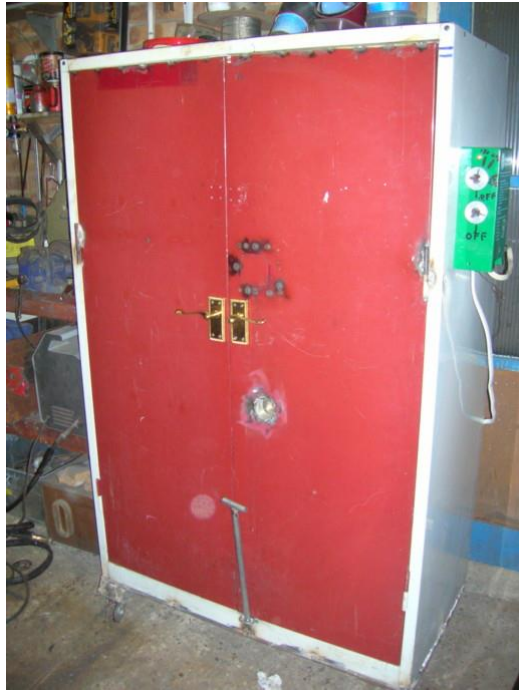
The finished oven with brass door handles. Below these in the right door is the thermometer.
