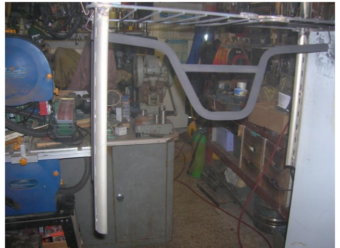
Powder coated and ready for the oven
