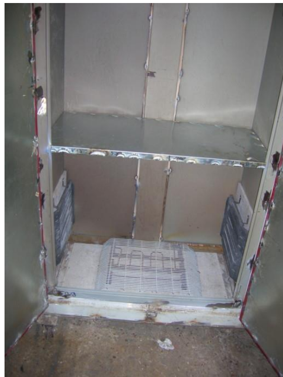
Inside, the three elements, the shelf is double skinned and insulated. When in place it cuts the oven area in half for better efficiency when all the height isn't needed, not perfect but it helps.
